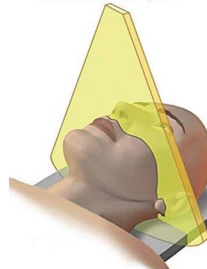
Fan Beam CT Used in 'conventional' Spiral CT
